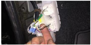
Connect the 3<sup>rd</sup> Brake light wiring (RED and BLACK) to the rear light cluster (See left hand image)
