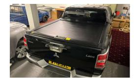
Pull the roller top back and ensure clearance with the tailgate. Then tighten side arms brackets.
