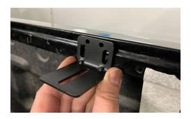
Fix the side brackets (measuring from the bulkhead) between 36-133 cm. These may need adjusting in height once the roller top is sat on the pick up tub.
