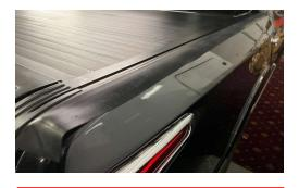
Side rubber may need heating to allow the seal to relax to the shape of the tub.
