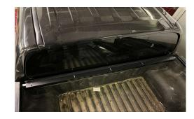
Fit the bulkhead bracket with the self tapping bolts supplied.
