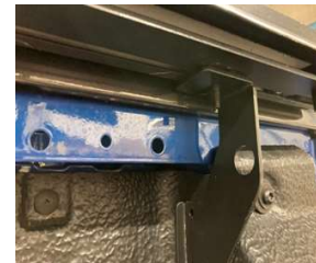
4. Assemble the Roller top, ensure joints between the bulkhead and side arms are sealed
