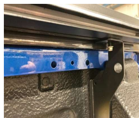
6. Fit the rear brackets (using the higher holes) adjust for the height of the vehicle tailgate and tighten
