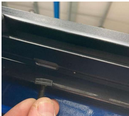
12. Slide the T-bolts into place
