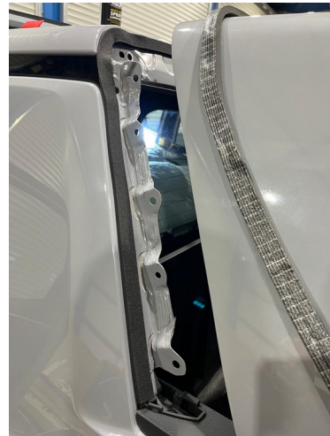
Use expanding foam along the base and bulkhead
