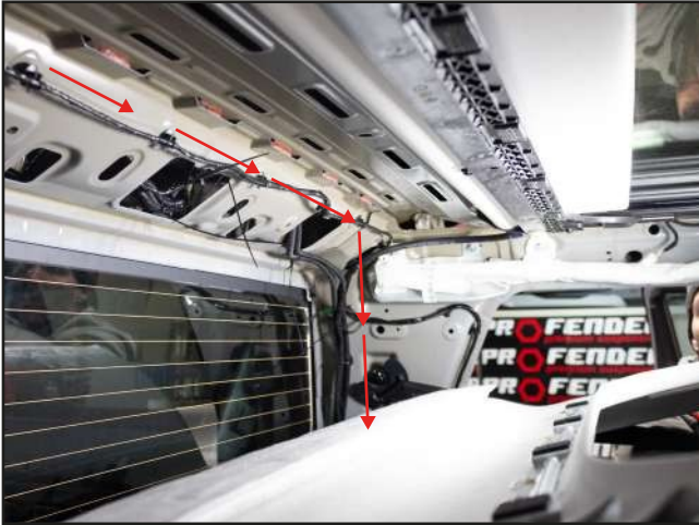
Feed Central locking wire down the left pillar
