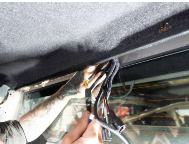
Feed wires into the canopy, connect break light and interior light. Use the heated rear window feed to connect in the canopy
