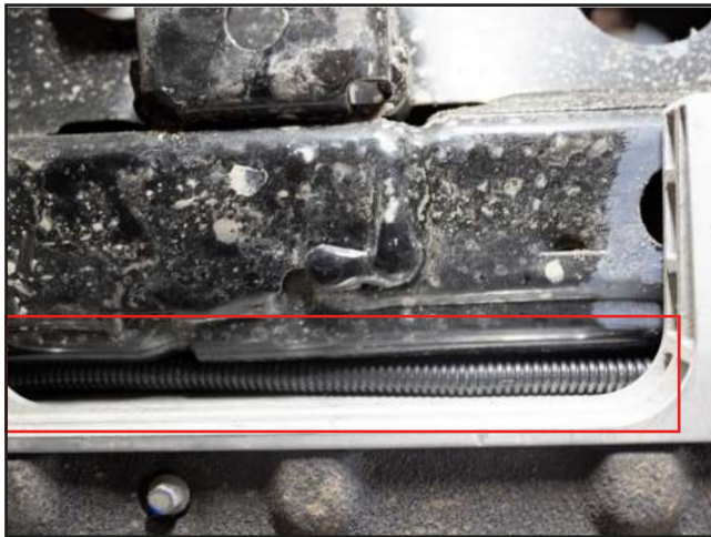
Feed Central locking wire down the left pillar
