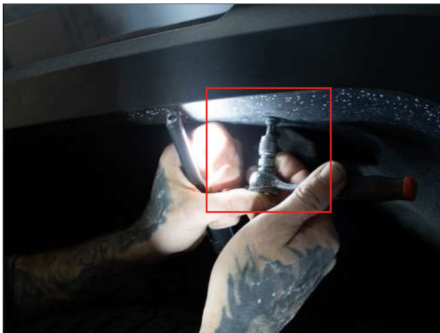
Remove left rear wheel arch for central locking wires
