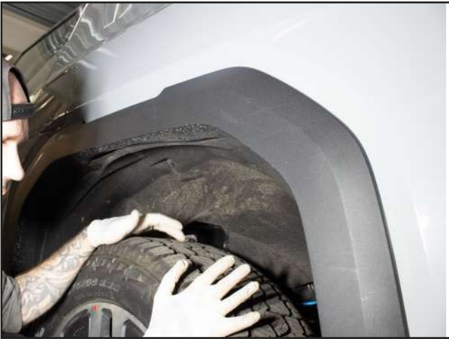
Remove left rear wheel arch for central locking wires
