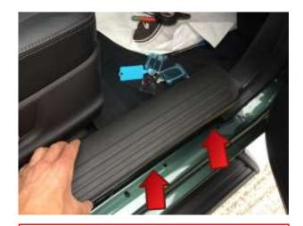
Ensure the ignition is off. Remove door sill trim from the driver's door, followed by the plastic trim in front of this (next to the accelerator pedals)
