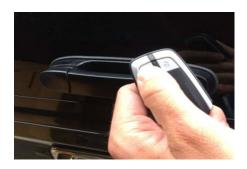
Check that the hardtop locks and unlocks using the vehicle's remote
