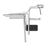
If the rails measured to be too close together, turn the screws counter clockwise.
