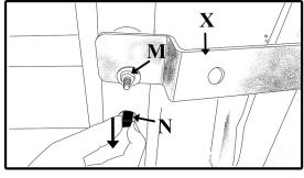
5.2 put main bracket (X) in position. Finger tighten nut M
