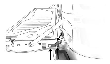
Pull the damper out and put damper bracket and tighten back the original bolt.
