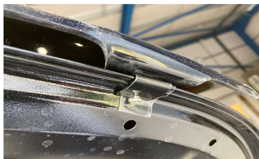
Fit outer brackets to Hilux and tighten bolts
