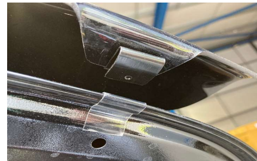
Fit two outer brackets to bonnet guard
