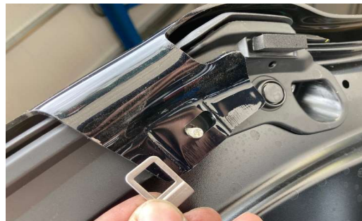
Add plate between Hilux and bonnet guard
