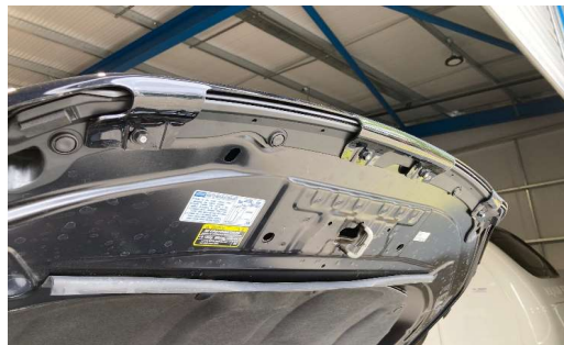
4 bolts fixed and tightened in place
