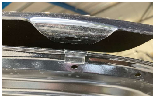
Fit protection tape where outer brackets will fit
