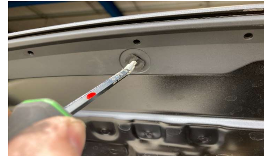
Screw bolts into plugs, holding the plug securely in place with a pliers
