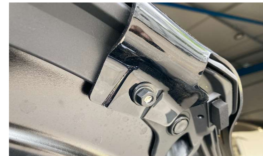
Fit washer and tighten nuts
