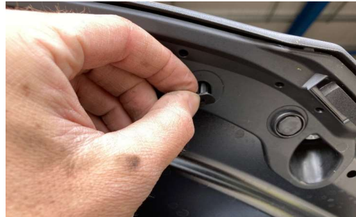
Insert new plugs into holes
